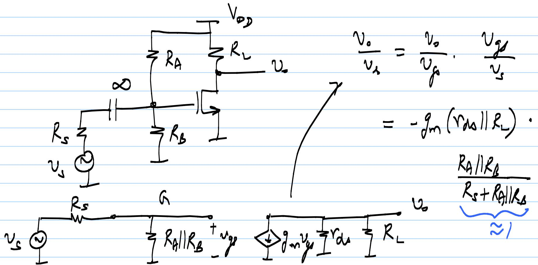
$$\frac{V_o}{V_s} \approx -g_m (r_{ds} || R_L) \quad \text{gain is smaller}$$
