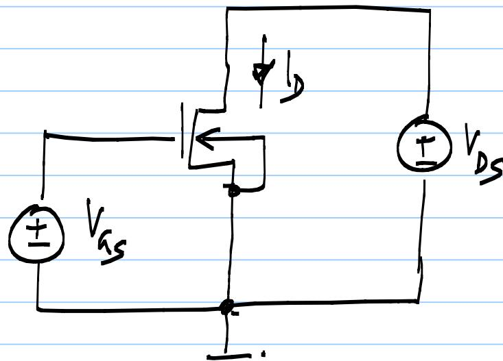
\* Try  $\frac{W}{L} = \frac{1.8\mu m}{0.18\mu m}, \frac{3.6\mu m}{0.36\mu m},$
