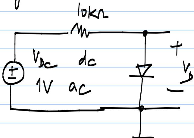
Sweep  $V_{DC}$  from  $1V$  to  $3V$
