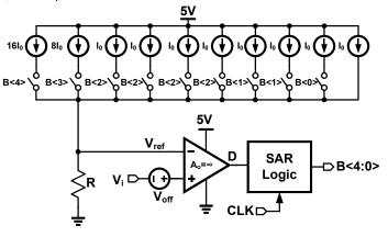
a) If V<sub>i</sub>=0.743V and V<sub>off</sub> = 0V, find D and B<4:0> every clock period till a final digital equivalent is found for the input.
