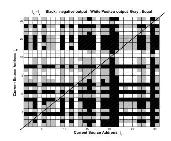
Fig. 10. Comparison of each cell current in upper segment with all other cell currents, a white box indicates that the current through the cell indicated on vertical axis is larger than the one on the horizontal axis. A black box indicates the opposite result.
