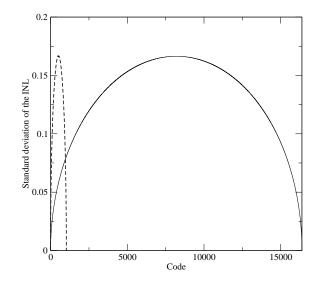
Fig. 2. The standard deviation of the INL at various codes for a 10 and 14 bit DAC
