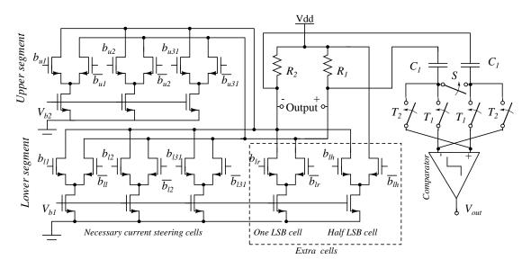
Fig. 5. Schematic of the segmented current steering architecture and error quantizer. Extra one LSB and half LSB cells have been added for error quantization
