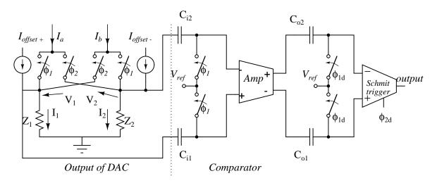
Fig. 6. Comparator used for DNL estimation
