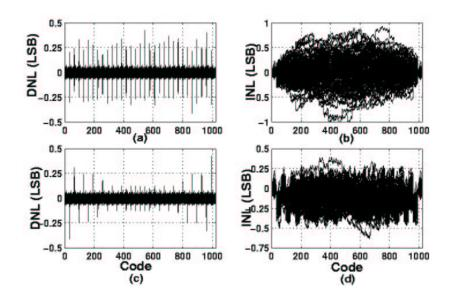
Fig. 4. DNL and INL from 100 MATLAB simulations for a 5+5 bit segmented DAC. (a) and (b) corresponding to the raw random sequence. (c) and (d) corresponding to modified sequence sorted using estimated DNL with 0.25LSB resolution. Note that the figure contains results from 100 simulations, so it appears that there are more than 32 transition points.
