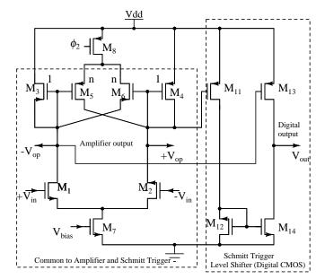
Fig. 7. Schematic of pre-amplifier(Amp), Schmitt trigger and level shifter
