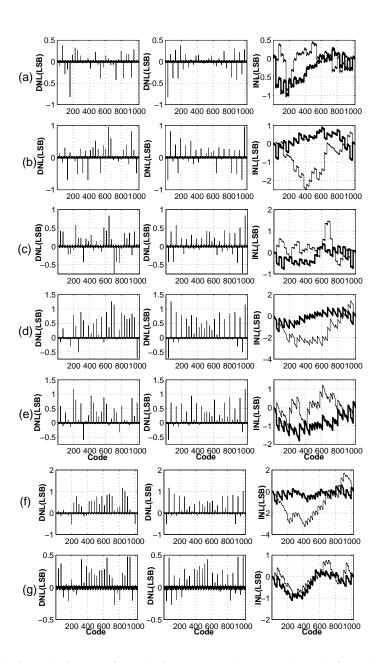
Fig. 12. DNL and INL before and after reconfiguration for seven samples. For each sample first column indicate DNL before reconfiguration, middle column indicate DNL after reconfiguration and INL before and after(thick line) reconfiguration in the last column respectively.
