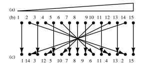
Fig. 1. Switching sequence mapping algorithm. (a) Error after sorting in ascending order (b) sequence of current source after sorting in ascending order and (c) sequence of current source after mapping.
