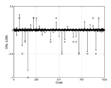
Fig. 11. DNL from external measurement and on-chip estimation. Continuous line with cross indicate DNL from external measurement, circle indicate DNL from on-chip estimation.
