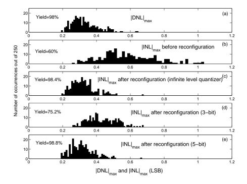
Fig. 3. Histogram of  $|DNL|_{max}$  and  $|INL|_{max}$  of a 5+5 bit DAC with  $\frac{\sigma I_L}{I_L} = 0.0208$  for 250 simulations. (a)  $|DNL|_{max}$ . (b)  $|INL|_{max}$  before reconfiguration. (c)  $|INL|_{max}$  after switching sequence optimization(infinite level quantization). (d)  $|INL|_{max}$  after switching sequence optimization(with 3-bit quantization levels). (e)  $|INL|_{max}$  after switching sequence optimization(with 5-bit quantization levels).
