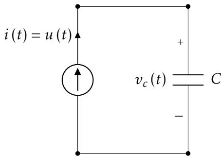
$$\begin{aligned} i(t) &= C \frac{dV}{dt} \\ \Rightarrow v_c(t) &= v_c(0) + \frac{1}{C} \int_0^t i(t) dt \\ v_c(t) &= \frac{t}{C} \end{aligned}$$
