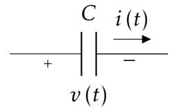
$q = CV$ , where \$V\$ is voltage drop across the capacitor
