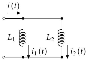
$$\begin{aligned} i(t) &= i_1(t) + i_2(t) \\ &= i_1(0) + \frac{1}{L_1} \int_0^t v(t) dt + i_2(0) + \frac{1}{L_2} \int_0^t v(t) dt \\ &= \sum_{k=1}^2 i_k(0) + \left( \frac{1}{L_1} + \frac{1}{L_2} \right) \int_0^t v(t) dt \end{aligned}$$
