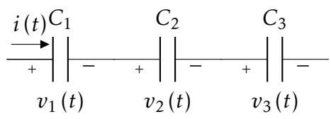
$$v_1(t) = v_1(0) + \frac{1}{C_1} \int_0^t i(t) dt$$
