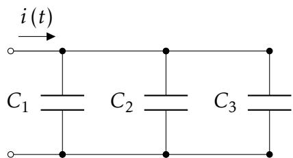
$$i(t) = C_1 \frac{dV}{dt} + C_2 \frac{dV}{dt} + C_3 \frac{dV}{dt}$$
