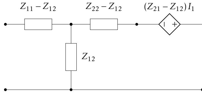
The above circuit is the equivalent T network for network  $N_1$ .
