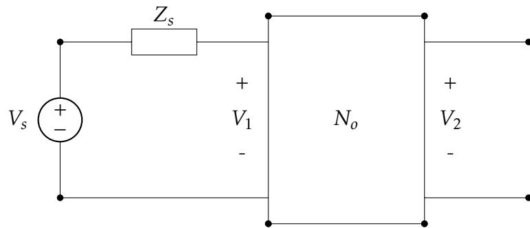
To find  $V_{oc}$  : Solve  $V_2$  when  $I_2 = 0$
