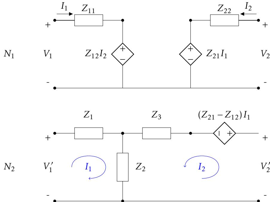
If we know the Y parameter of a network then we represent the network as a  $\pi$  or  $\Delta$  network. Similarly using Z parameter we can represent the network as a T network. Find Z<sub>1</sub>, Z<sub>2</sub> and Z<sub>3</sub> so that the two networks have the same characteristics at the two ports i.e if we connect current sources I<sub>1</sub> and I<sub>2</sub> at the ports, the corresponding voltages should be identical.
