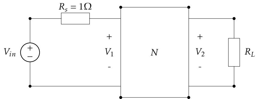
Find zero input and zero state response, output =  $V_2$  and  $V_{in} = u(t)$
