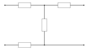
In above picture "rectangles" represents the components and the "solid lines" represents the connecting wires. In order to analyse the system, we need I-V characteristics of all components. As our aim is to find out the response (voltage across the component or current through the component) using the component models for a given excitation.
