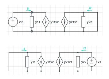
If  $y_{12} = y_{21}$ ;  $i_1 = i_2$ . Can interchange the position of the voltage source and the point at which current is measured.
