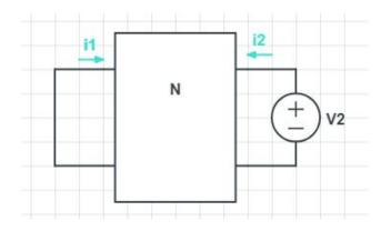
$y_{12}, y_{22}$  are calculated by setting  $V_1 = 0$  i.e shorting the input port, adding voltage source at the output port and finding  $I_1, I_2$ .
