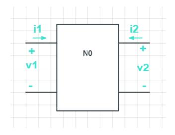
First we choose  $V_1, V_2$  as inputs and  $I_1, I_2$  as outputs and set  $\begin{bmatrix} I_1 \\ I_2 \end{bmatrix} = \begin{bmatrix} y_{11} & y_{12} \\ y_{21} & y_{22} \end{bmatrix} \begin{bmatrix} V_1 \\ V_2 \end{bmatrix}$ Measure the Y parameters as follows.
