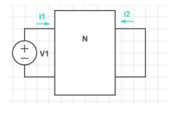
$y_{11} = \frac{I_1}{V_2}|_{V_2=0}$  $y_{21} = \frac{I_2}{V_2}|_{V_2=0}$
