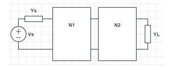
If we have cascaded networks,  $y_{in_2}$  will be the load admittance for  $N_1$ . HW: Find the overall gain of the cascaded networks.
