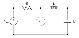
$$V_{in} = iR + L\frac{di}{dt} + \frac{1}{C}\int idt$$
