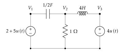
Use initial value theorem and find  $v_2(0^+)$  from  $V_2(s)$  and final value theorem to find  $\lim_{t\to\infty} v_2(t)$
