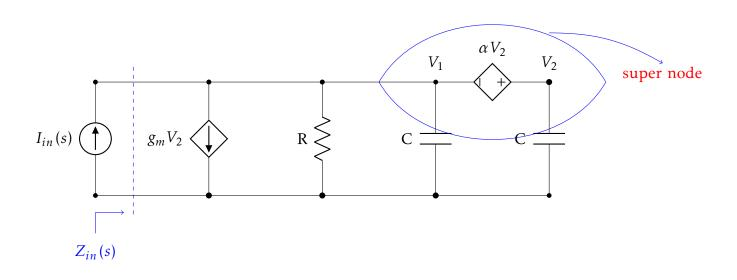
$$V_1\left(\frac{1}{R} + sC\right) + V_2(sC) + V_2g_m = I_{in}(s)$$
