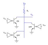
Open collector buffers: One of the inputs drives the bus. The input to all other gates should be adjusted so that the corresponding outputs are high (i.e. turn OFF the output transistors).
