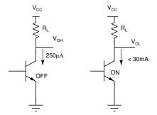
Note the current direction is into the gate for both output high and low voltages. The value of the resistor should be adjusted so that we get valid high and low voltages.
