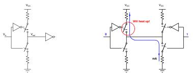
When output is high, typical current  $400\mu$ A. The current is 10s of mA when output is low. In the worst case, could destroy one of the switches if outputs are connected together. Voltage could be at an intermediate level and cannot be interpreted as a 0 or 1.
