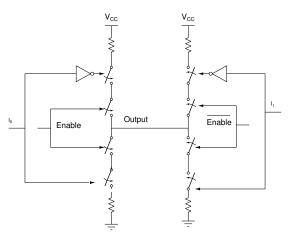
Can connect multiple gates to a common bus and enable only one at a time
