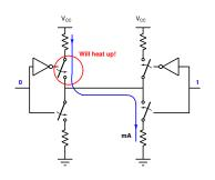
When output is high, typical current  $400\mu\text{A}$ . The current is 10s of mA when output is low. In the worst case, could destroy one of the switches if outputs are connected together.
