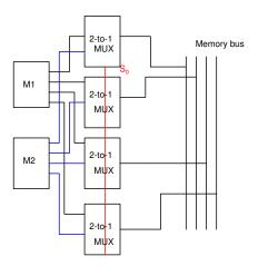
Can use several 2-to-1 MUXes to route one of the inputs to the output.
