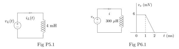
6. The voltage at the terminals of the 300  $\mu$ H inductor is as shown in Fig P6.1. The inductor current is known to be zero for  $t \leq 0$ .
