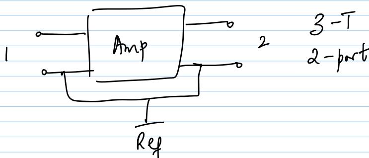
$$\left. \begin{array}{l} I_1 = f_1(v_1, v_2) \\ I_2 = f_2(v_1, v_2) \end{array} \right\} \text{Use a } 2-\text{D Taylor Series}$$
