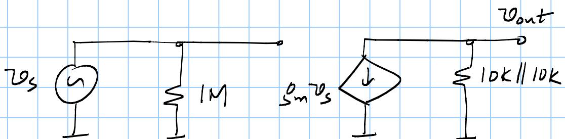
$$\text{Incremental gain} = \frac{V_{out}}{V_s} = -\text{gm} (5 \text{ k})$$
