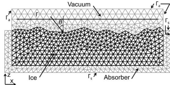
Figure 1: Finite element mesh showing vacuum-air interface and an incident radar wave of wavelength,  $\lambda= 2.17$  cm. The horizontal extent of ice is  $70\lambda$ , and the average depth is  $3.5 \lambda$ .
