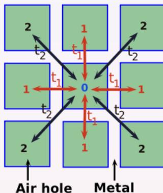
Schematic of the interaction process between the scattered field from the lattice sites: interaction only up to second nearest neighbor is shown. The interaction path/ the arrows are drawn along the direction of the lattice vector. The numbers on the neighboring holes denote their distances from the  $0^{th}$  hole. Here,  $t_1$  and  $t_2$  denote the hopping parameters.
