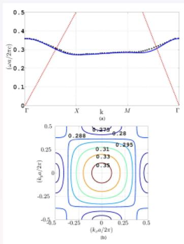
Second band of dielectric PhC (dimension is same as that of the super-collimating structure, except that the  $\text{SiO}_2$  undercladding is absent here). The black circles correspond to the FDTD results obtained by J. Witzens et al. (*IEEE J. of Selected topics in Quantum Elec.* **8** 1246, 2002). FDTD results predicted a flat contour at  $0.295(c/a)$ .
