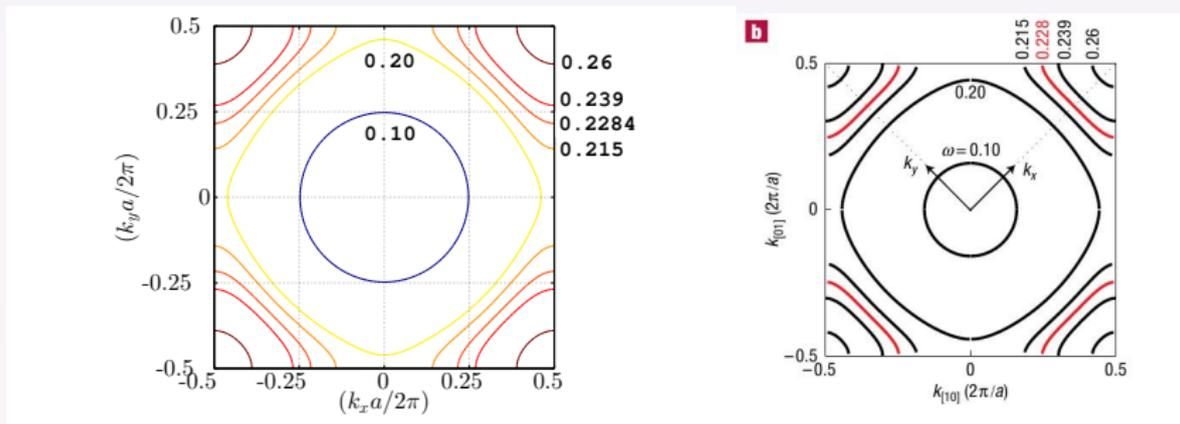
**Figure:** Contour plot for the first band of the super-collimating photonic crystal. Left: predicted by tight binding model. Right: FDTD simulation [P. T. Rakich et al., *Nature Materials* **5**, 93, 2006].
