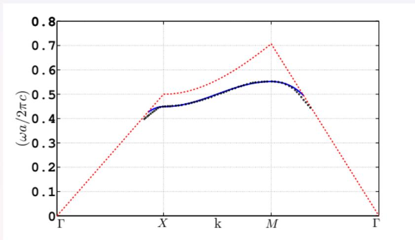
**Figure:** This is what we plot! Ignore the black circles for the time being. The blue line shows the band-diagram and the red dotted line is light-line.
