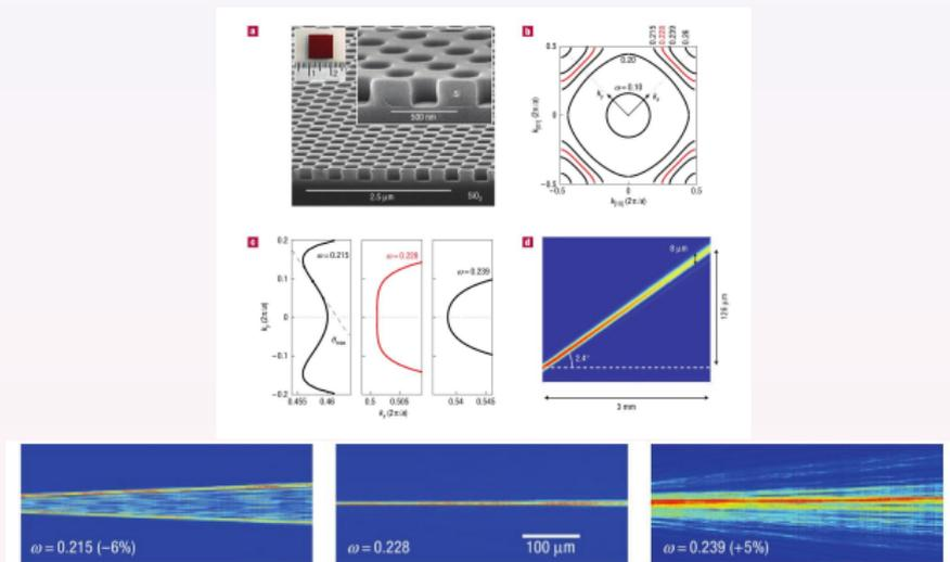
Figure: Super-collimation in PhC.  $a = 350 \text{ nm}$ ,  $r = 0.3a$  [P. T. Rakich et al., *Nature Materials* **5**, 93, 2006].
