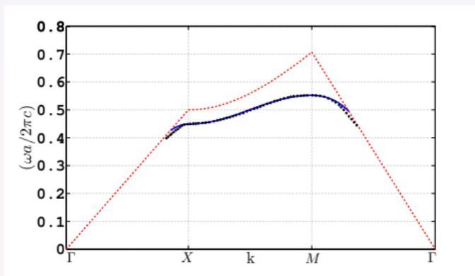
High frequency limit band diagram of surface wave on a 2D array of square holes of infinite depth drilled on PEC. For each hole, the each side,  $b = 0.875a$ . Blue/solid line: dispersion diagram obtained using our theory, black circles: dispersion diagram obtained by FDTD (refer to M. Qiu, *Opt. Express* **13** 7583, 2005) . Red/dashed line: light line.
