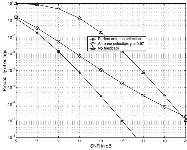
Fig. 4: SNR vs. Probability of outage for  $4 \times 2$  system, normalized Doppler = 0.06
