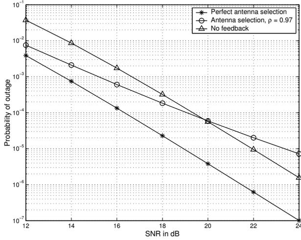
Fig. 3: SNR vs. Probability of outage for  $2 \times 2$  system, normalized Doppler = 0.06
