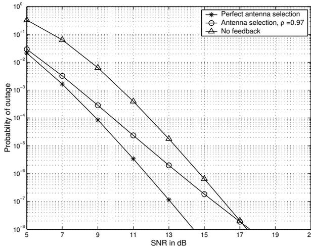
Fig. 5: SNR vs. Probability of outage for  $2 \times 4$  system, normalized Doppler = 0.06
