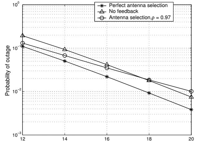
Fig. 2: SNR vs. Probability of outage for  $2 \times 1$ , normalized Doppler = 0.06
