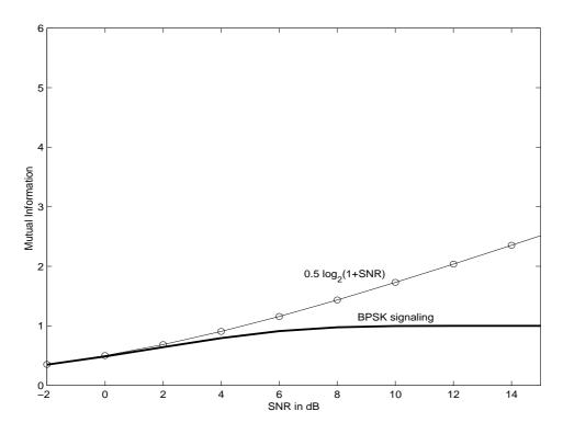
Figure 2: Mutual Information for BSPK signaling vs. SNR
