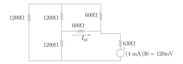
Figure 6: (Problem 2) Incremental network for  $R_x = 630\Omega$
