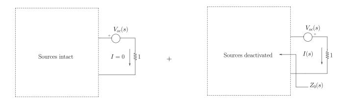
Figure 5: (*Problem 1(b)*) Applying the superposition principle
