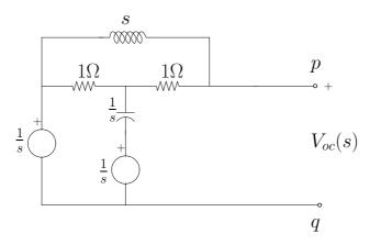
Figure 1: (Problem 1(a)) Laplace-transformed network
