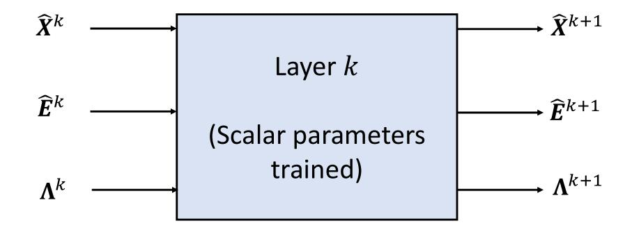
One iteration of ADM algorithm is one layer
