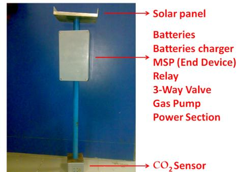
Figure 3: A CO<sub>2</sub> sensing WSN node.
