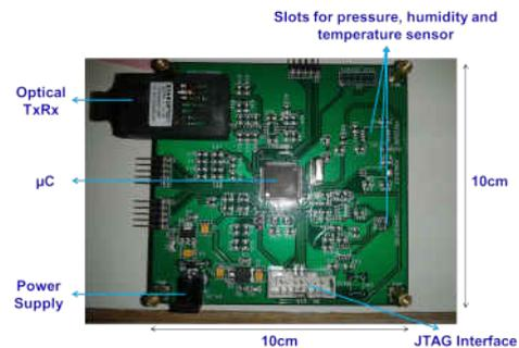
Figure 3: The MSP based prototype.
