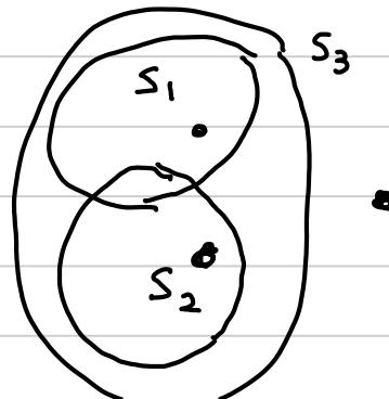
$$\begin{aligned} S_1 : & R_1 \leq I(X_1; Y | X_2) \\ S_2 : & R_2 \leq I(X_2; Y | X_1) \\ S_3 : & R_1 + R_2 \leq I(X_1, X_2; Y) \end{aligned}$$
