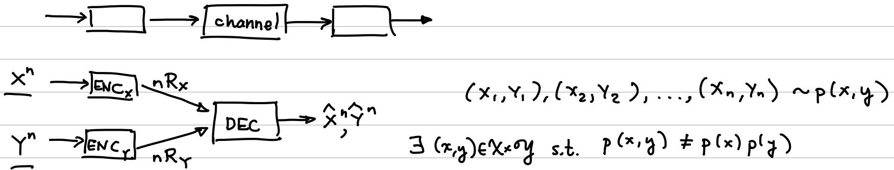
A multiple access source code is defined by a pair of encoders
