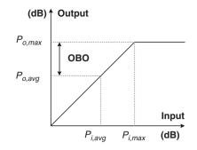
Figure 2.14. Output back-off point of power amplifier
