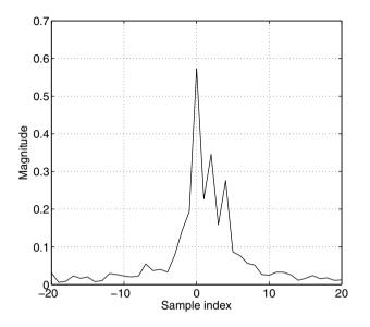
Figure 5.9. Resolved channel profile from a matched filter output
