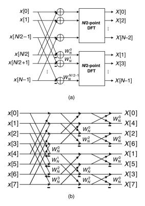
**Figure 9.2.** (a) Signal flow graph of radix-2 decimation-in-frequency decomposition and (b) its application in 8-point DFT computation
