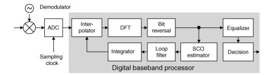
Figure 5.15. OFDM baseband receiver architecture with time-domain sampling clock offset compensation using an interpolator
