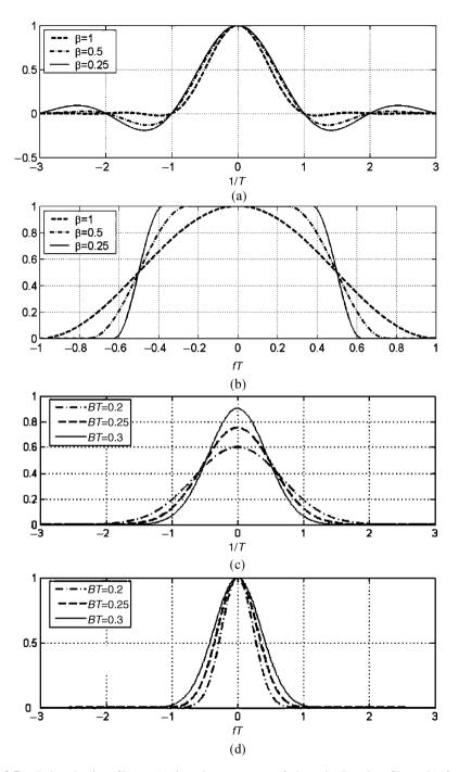
**Figure 2.7.** Pulse-shaping filters: (a) impulse response of the raised-cosine filter, (b) frequency response of the raised-cosine filter, (c) impulse response of the Gaussian filter and (d) frequency response of the Gaussian filter
