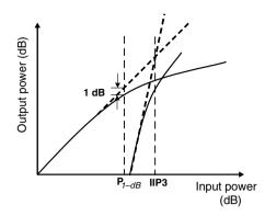
Figure 4.12. Illustration of PA nonlinearity
