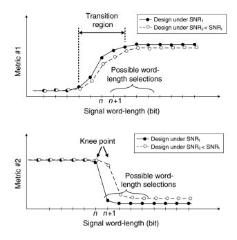
Figure 8.23. Performance characteristics used for signal word-length selection
