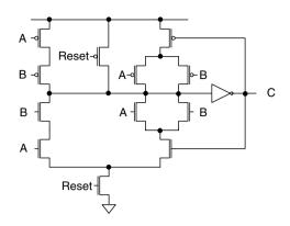
Figure 9.17. Circuit diagram of the C-element
