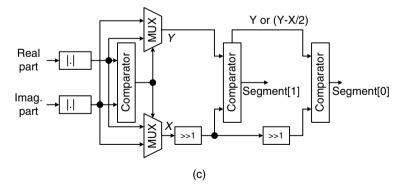
**Figure 9.29.** Circuits of (a) two-segment vector magnitude linear approximation, (b) four-segment vector magnitude linear approximation and (c) general vector mapping to the first octant and segment identification
