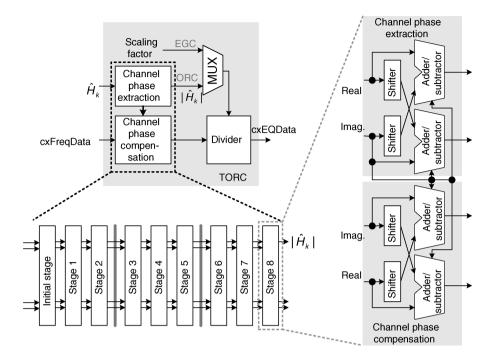
Figure 10.4. Block diagram of TORC equalization. Reproduced by permission of © 2005 IEEE
