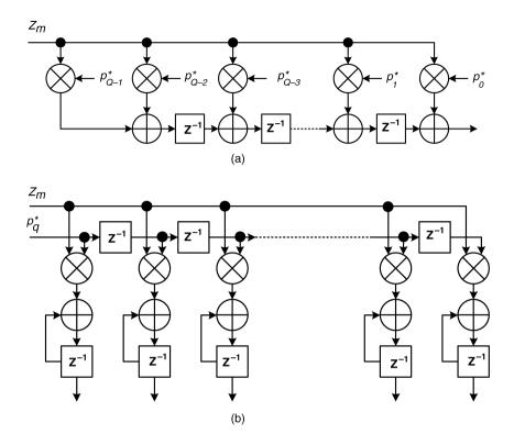
Figure 5.10. (a) Architecture of the transposed matched filter and (b) architecture of the correlator bank
