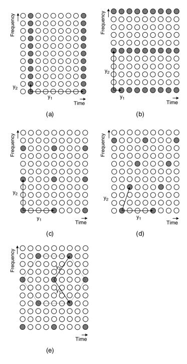
**Figure 6.1.** Illustrations of several common pilot patterns: (a) block type, (b) comb type, (c) rectangular grid, (d) parallelogram-shaped grid and (e) hexagonal grid
