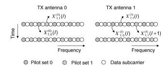
Figure 7.6. Space-frequency pilot insertion in MIMO-OFDM systems
