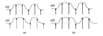
**Figure 4.8.** (a) Sampling error occurs when the baseband transmitted signal x(t) and the baseband received signal z(t) are sampled at different clock rates. (b) Baseband received signal z(t) is expanded due to the Doppler effect, resulting in sampling error, even without clock rate mismatch
