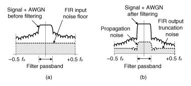
**Figure 8.20.** Illustration of the noise floor changes due to filtering (a) noise before filtering and (b) noise after filtering
