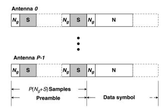
Figure 7.4. Preamble design for MIMO–OFDM systems
