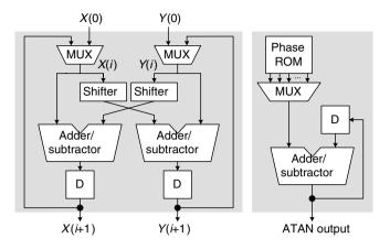
Figure 9.24. Basic CORDIC rotation stage and angle accumulator
