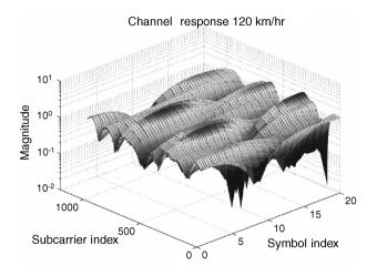
Figure 6.10. Time-varying channel frequency response
