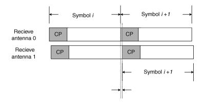
Figure 7.7. Symbol timings of different receive branches in MIMO-OFDM systems
