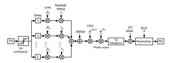
Figure 4.13. Equivalent baseband channel model
