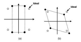
**Figure 4.10.** IQ imbalance effect on QPSK signals: (a) gain error in LO signals, (b) phase error in LO signals
