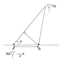
Figure 4.4. Illustration of a signal reception under the Doppler effect
