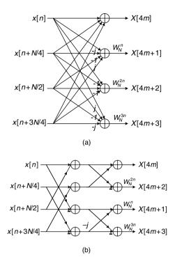
**Figure 9.3.** (a) Radix-4 butterfly and (b) radix- $2^2$  butterfly
