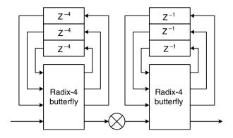
Figure 9.11. Radix-4 single-path delay feedback (N = 16)
