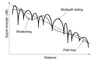
Figure 4.1. Illustration of path loss, shadowing and multipath fading
