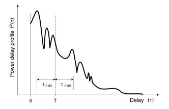
Figure 4.2. Typical multipath channel power delay profile
