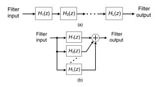
**Figure 8.21.** Practical IIR filter implementation: (a) cascade form and (b) parallel (poly-phase) form, where  $H_1(z), H_2(z), \ldots, H_L(z)$  are first-order or second-order filters
