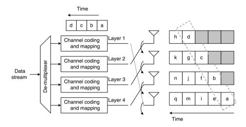
Figure 7.9. D-BLAST spatial multiplexing transmission
