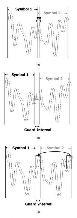
**Figure 2.11.** (a) Illustration of ISI due to multipath delay; (b) zero-padding guard interval to avoid ISI; (c) guard interval with cyclic prefix to eliminate ISI and ICI
