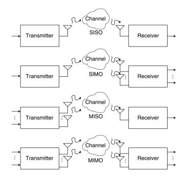
Figure 7.1. Illustration of transmitters/receivers with different antenna configurations
