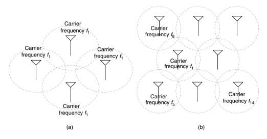
Figure 1.1. (a) Single-frequency network and (b) multi-frequency network
