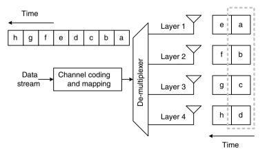
Figure 7.10. V-BLAST spatial multiplexing transmission
