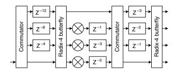
**Figure 9.9.** Radix-4 multi-path delay commutator FFT architecture (N = 16)
