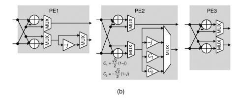
Figure 9.12. (a) Variable-length FFT processor and (b) its processing elements
