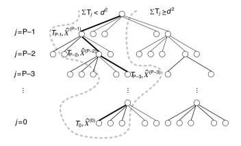
Figure 7.12. Tree-search architecture in sphere decoder
