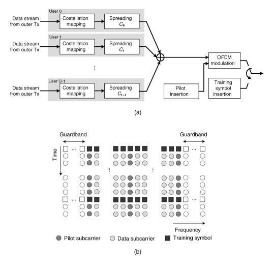
**Figure 10.1.** (a) Block diagram of the MC-CDMA baseband transmitter (reproduced by permission of © 2005 IEEE) and (b) allocation of pilot subcarriers and training symbols
