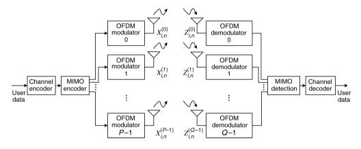
Figure 7.3. A MIMO–OFDM system with P transmit antennas and Q receive antennas
