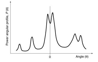
Figure 4.6. A typical signal power angular profile
