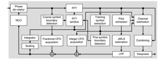
Figure 10.2. Block diagram of the MC-CDMA receiver. Reproduced by permission of  $\odot$  2005 IEEE
