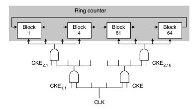
Figure 9.19. Clock driver tree and gating signal
