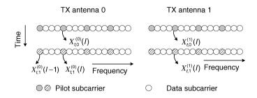
Figure 7.5. Space-time pilot insertion in MIMO-OFDM systems
