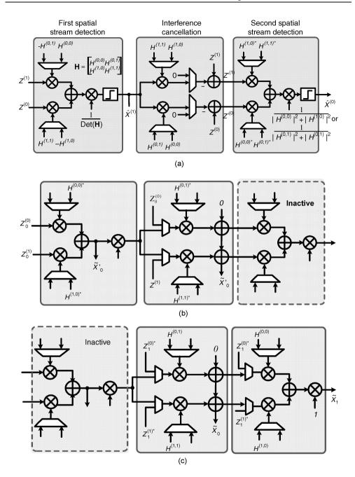
**Figure 10.9.** Configurations of the proposed MIMO detector working (a) as the VBLAST detector, (b) as the STBC decoder (first phase) and (c) as the STBC decoder (second phase)
