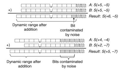
Figure 8.13. Binary addition of two fixed-point numbers
