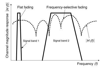
Figure 4.3. Channel frequency response and signal bands for flat fading and frequency-selective fading
