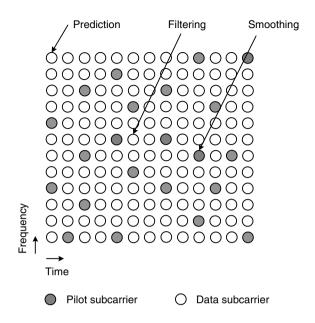
Figure 6.9. Arbitrary sampling grid used in a two-dimensional MMSE interpolator for smoothing, filtering and prediction
