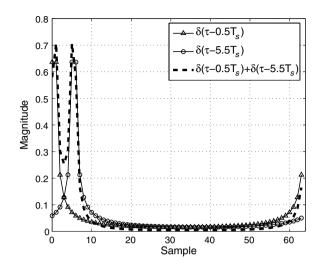
Figure 6.3. Energy leakage in discrete-time channel impulse magnitude response
