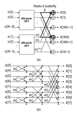
**Figure 9.1.** (a) Signal flow graph of radix-2 decimation-in-time decomposition and (b) its application in 8-point DFT computation
