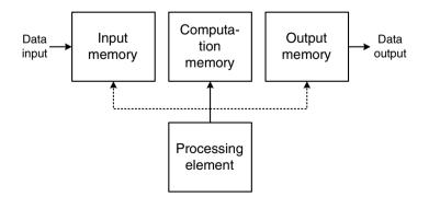
Figure 9.5. Memory-based FFT architecture
