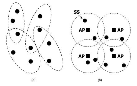
Figure 1.4. (a) Scatter network and (b) cellular network
