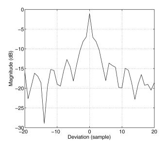
Figure 5.8. Impulse-like auto-correlation function of the long preamble in the IEEE 802.16e-2005 OFDM mode
