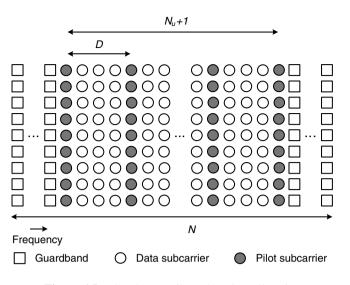
Figure 6.5. Comb-type pilot subcarriers allocation
