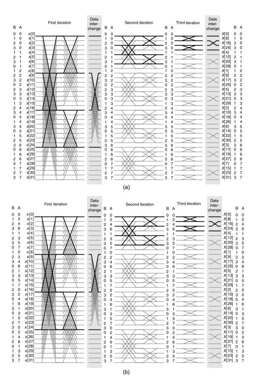
Figure 9.7. Signal flow graph of a 32-point FFT for the memory-based architecture: (a) normal addressing mode and (b) alternative addressing mode
