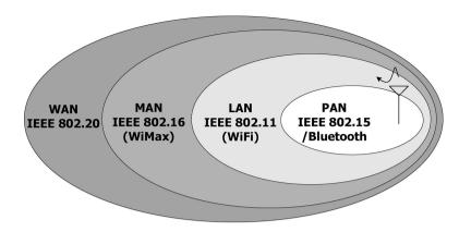
Figure 1.3. Illustration of several IEEE wireless network standards
