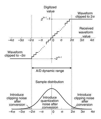
Figure 8.4. Dynamic range mapping of the ADC input signal
