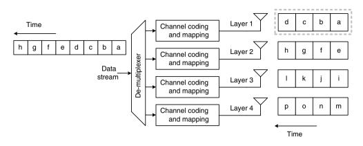
Figure 7.11. H-BLAST spatial multiplexing transmission
