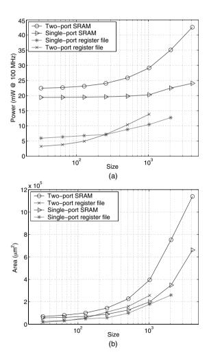
Figure 9.20. (a) Simulated power and (b) simulated area of several delay buffers using different approaches
