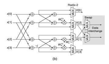
Figure 9.6. (a) Conflict-free addressing mixed-radix FFT processor and (b) radix-4/2 butterfly unit
