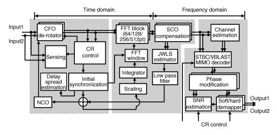
Figure 10.8. Architecture of the CR baseband receiver
