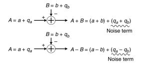
Figure 8.12. Propagation error model of a fixed-point adder/subtractor
