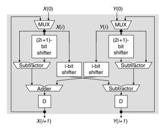
Figure 9.27. Scaling-free CORDIC micro-rotation stage
