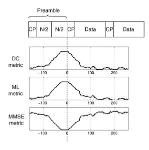
Figure 5.5. Waveforms in three symbol timing detection algorithms
