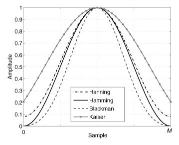
Figure 2.8. Windowing functions
