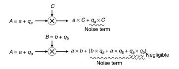
Figure 8.14. Propagation error model of fixed-point multipliers
