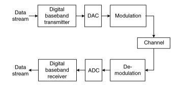
Figure 5.1. Block diagram of a simplified wireless communication system
