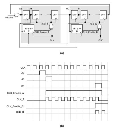
Figure 9.16. (a) Ring counter with clock gating by R-S flip-flop and (b) its timing diagram
