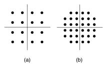
**Figure 2.3.** Signal constellations of two quadrature amplitude modulation techniques: (a) 16-QAM and (b) 32-QAM
