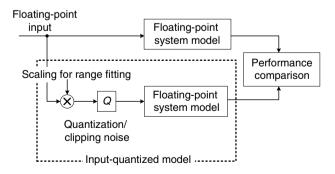
Figure 8.22. Input-quantized model and its performance evaluation
