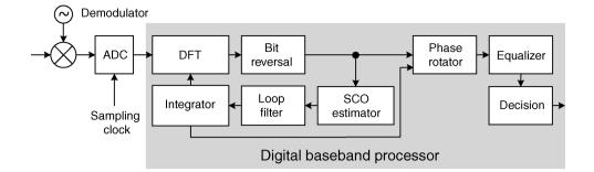
**Figure 5.17.** OFDM baseband receiver architecture that uses the frequency-domain phase rotator for SCO compensation
