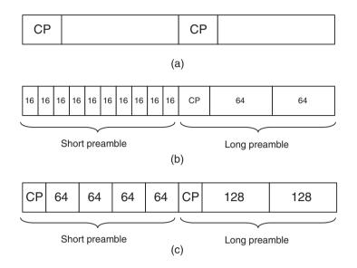
**Figure 5.4.** Time-domain periodic repetitions in (a) general OFDM symbols, (b) preambles of IEEE 802.11a and (c) preambles of IEEE 802.16e-2005 OFDM mode
