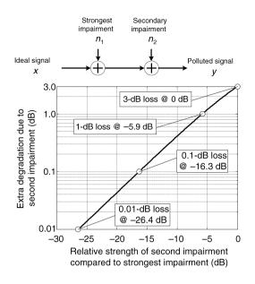
Figure 8.2. SINR degradation from a secondary impairment
