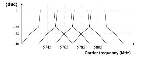
Figure 2.12. Spectrum mask for wireless LAN signal in the U-NII band
