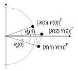
Figure 9.23. Trajectory of the vector during the CORDIC process using the angle accumulation mode
