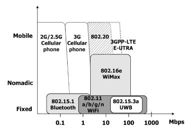
Figure 1.5. Mobility versus transmission rate of several wireless communication standards
