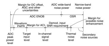
Figure 8.10. Dynamic range budget for ADC precision requirement estimation
