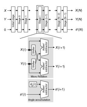
Figure 9.25. Parallel implementation of several CORDIC micro-rotation stages
