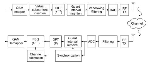
Figure 2.16. Typical OFDM transceiver architecture
