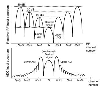
Figure 8.9. ACI conditions at the receiver front-end and ADC input
