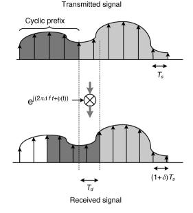
Figure 5.2. Synchronization errors in OFDM baseband signals
