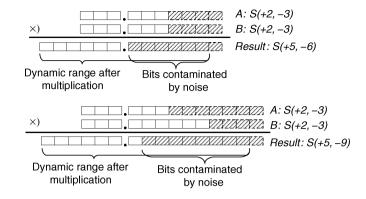
Figure 8.15. Binary multiplication of two fixed-point numbers
