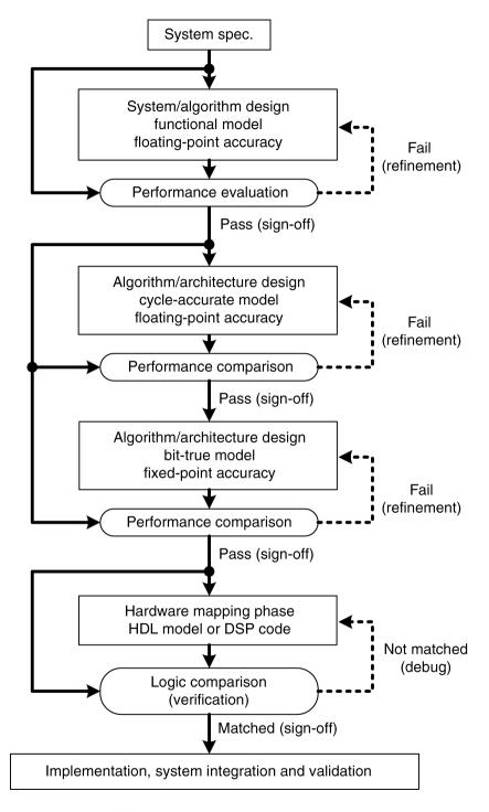
Figure 8.1. System design flow illustration
