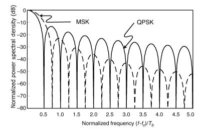
Figure 2.6. Power spectral density functions of QPSK and MSK signals
