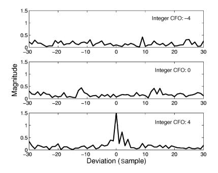
Figure 5.11. Matched filter output waveforms for three different values of integer CFO when the received signal suffers an integer carrier frequency offset of  $+4f_S$
