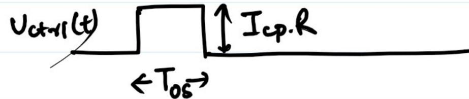
$$V_{ctrl} = \sum_{n=1}^{\infty} \frac{2I_{cp} \cdot R}{n\pi} \sin\left(n\pi \frac{T_{os}}{T_R}\right) \cos(n\omega_R t)$$
