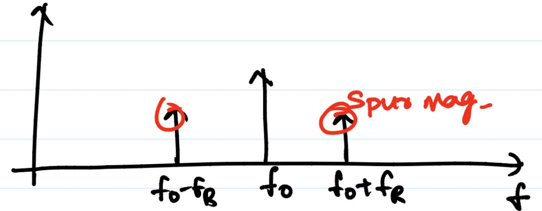
$$\text{Spur mag. (in dB)} = 20 \log \left( \frac{F_{BW}}{2F_R} \cdot \Delta\phi_{os} \right) - \underbrace{20 \log \left( \frac{N_R}{N_{p3}} \right)}_{\text{Ref. spur suppression}}$$
