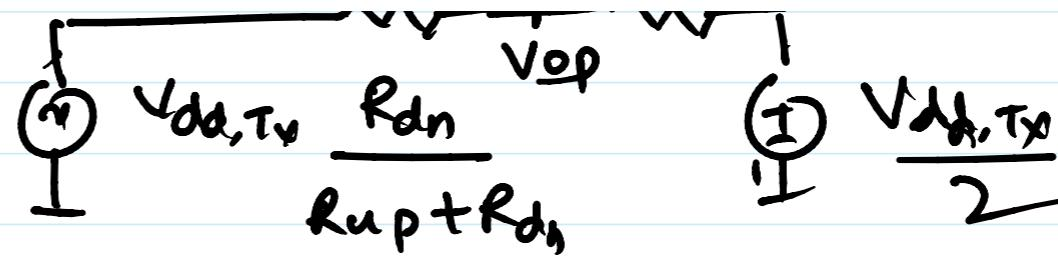
$$V_{op} = \frac{R_T}{R_T + R_{up} \parallel R_{dn}} \underbrace{\frac{V_{dd,Tx}}{R_{dn}}}_{R_{up} + R_{dn}} + \underbrace{\frac{R_{up} \parallel R_{dn}}{R_T + R_{up} \parallel R_{dn}} \frac{V_{dd,Tx}}{2}}$$
