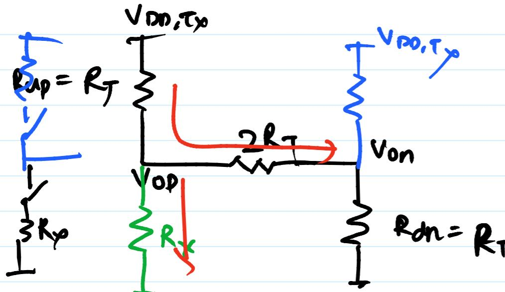
$$V_{op} = \frac{3}{4} V_{DD,Tx}$$
