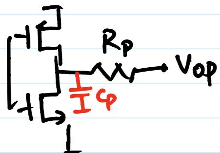
$$R_{PMOS} + R_P = R_{NMOS} + R_{P2} = R_T \quad (\text{Typ. } 27^\circ\text{C, 1V})$$
