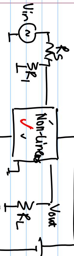
$$V_{out} = f(V_{in}) = \alpha_0 + \alpha_1 V_{in} + \alpha_2 V_{in}^2 + \dots$$
