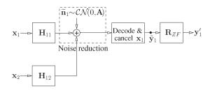
Fig. 7. Sequence of operations to show the decodability of  $W_{22}$  at receiver 1 in the MIMO ZC.
