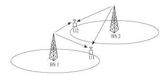
Fig. 1. Illustration of the X channel communication model in the cellular downlink.
