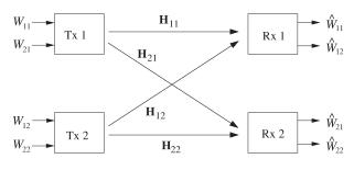
Fig. 2. MIMO X channel.
