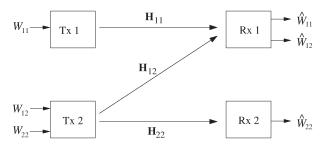
Fig. 3. MIMO Z channel.
