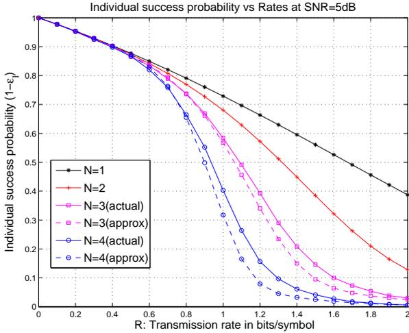
Fig. 4. Success probability  $1 - \tilde{\varepsilon}_i(N)$  versus the transmission rate  $R$  for different number of users. Here  $\gamma = \sqrt{10}$  (5dB) and we assume that all the users transmit at the same rate.
