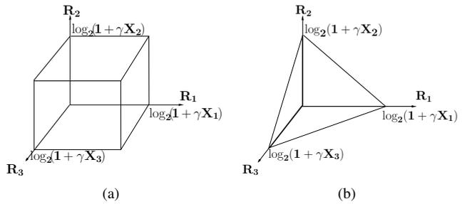
Fig. 2. High and low SNR approximations of a 3 user MAC capacity region.
