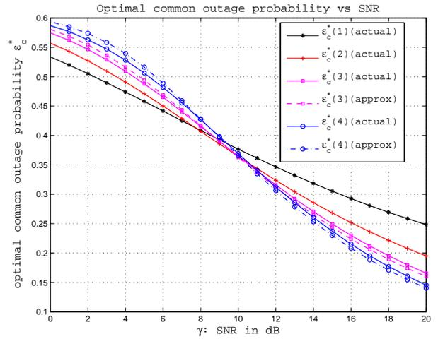
Fig. 5. Optimal common outage probability that maximizes the goodput versus the SNR for different  $N$ .
