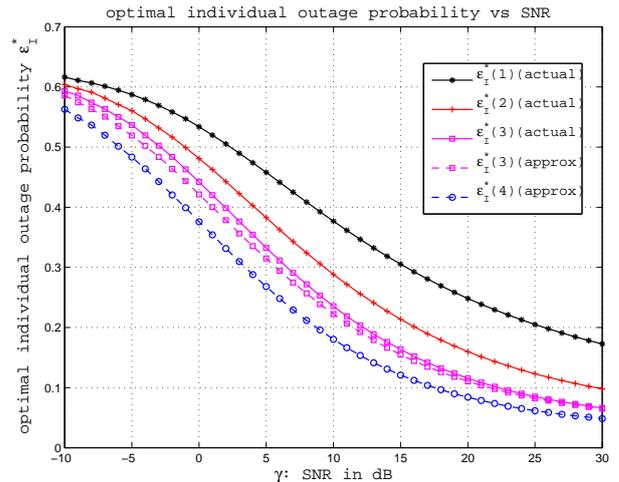
Fig. 6. Optimal individual outage probability that maximizes the goodput versus the SNR for different  $N$ .
