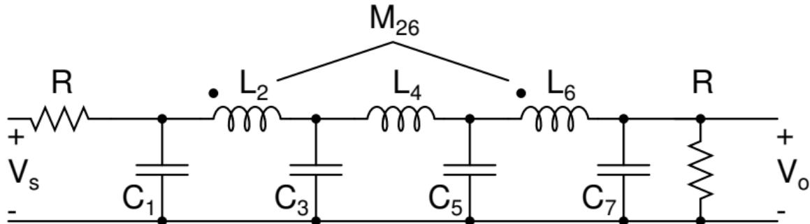
$$\frac{V_o(s)}{V_s(s)} = \frac{1 - s^2(C_3 + C_5)M_{26} - s^4C_3C_5L_4M_{26}}{D_7(s)}$$
