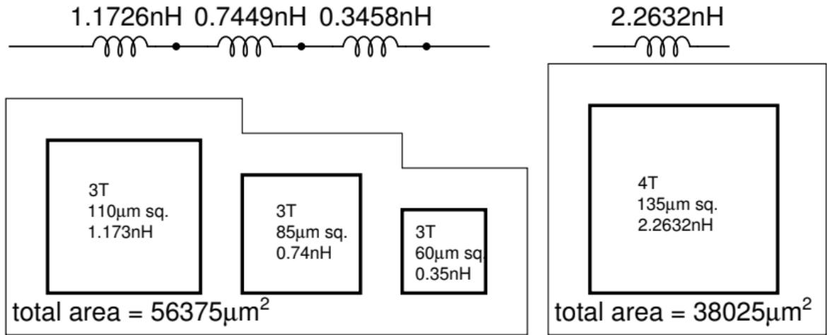
\* The area of the single spiral is incorrectly given as 27225 $\mu\text{m}^2$  in the paper
