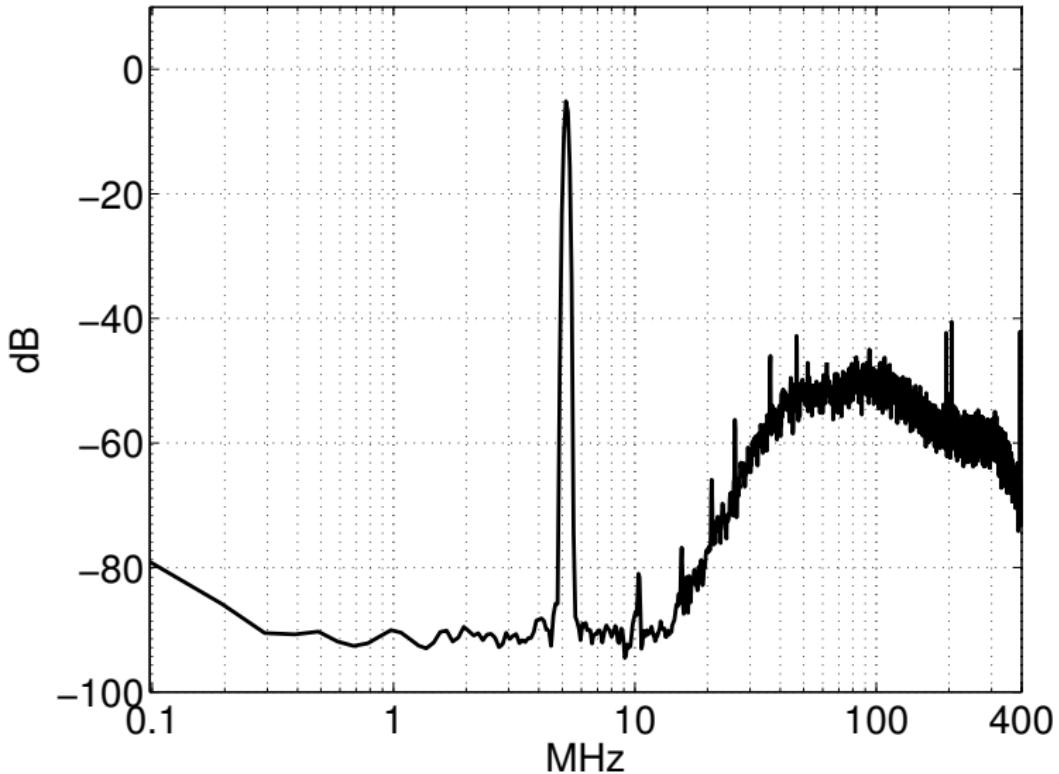
*Output spectrum;  $HD_2 = -76 \text{ dB}$   $HD_3 = -72 \text{ dB}$*
