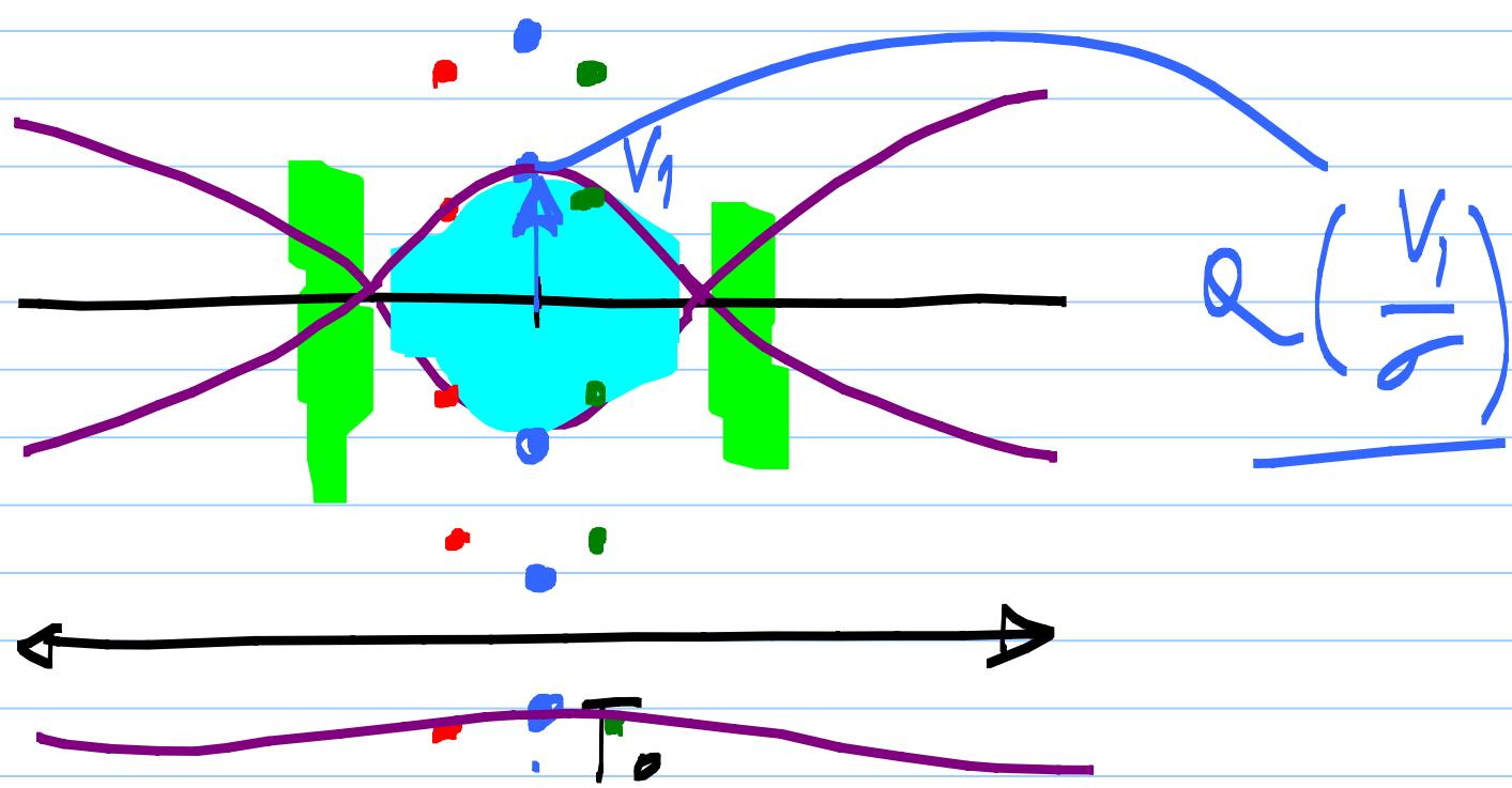
Horizontal eye opening: clock timing jitter
