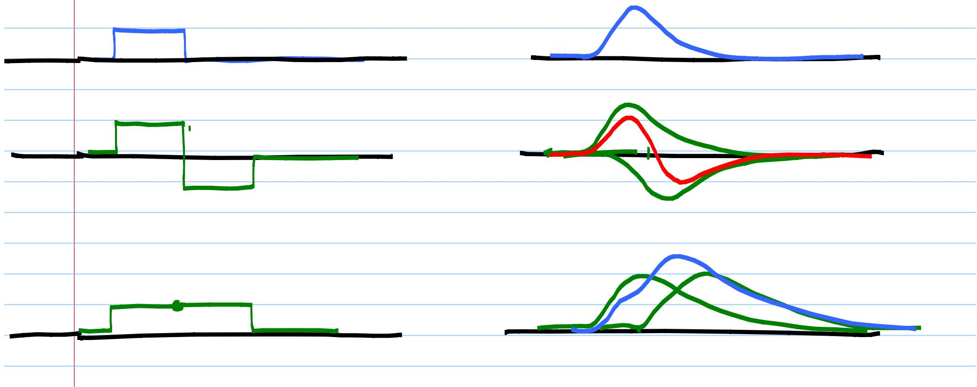
Output waveform in each symbol interval is a result of multiple bits. Waveforms depends on the bit pattern.
