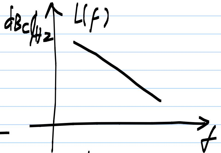
Ring oscillator has a higher phase noise than LC oscillator
