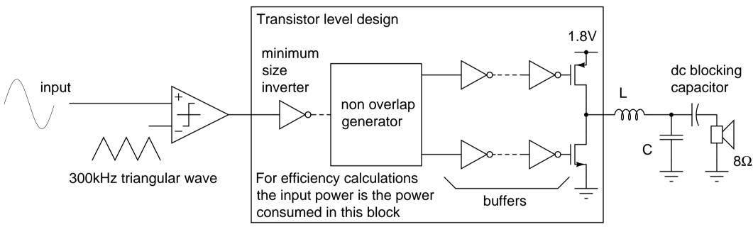
(dc blocking capacitor not required for bridged three level topology)
