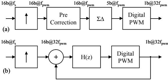
Figure 8. Digital PWM (a) pre-correction (b) PWM- $\Sigma\Delta$ .
