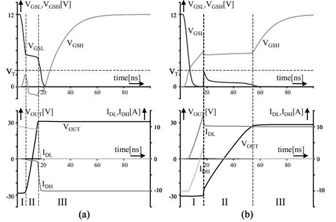
Figure 13. Rising output transition (a) soft switching (b) hard switching.
