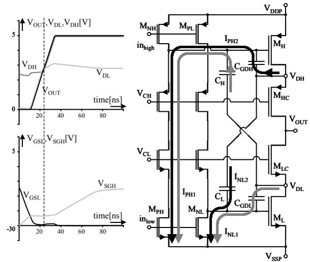
Figure 17. Cascoded class-D output stage for direct battery hookup.
