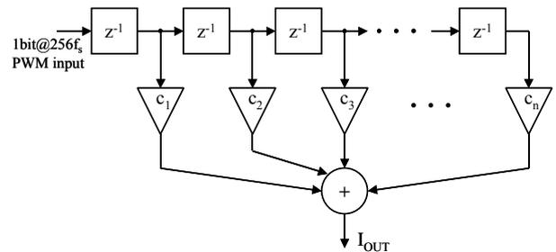
Figure 20. FIRDAC block diagram
