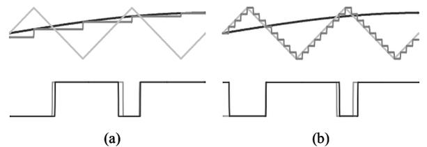
Figure 7. Digital PWM (a) sampling (b) quantization.
