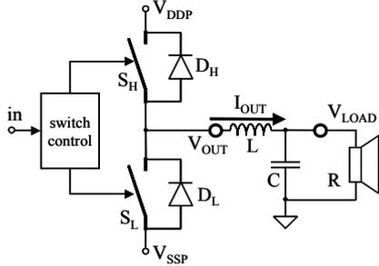
Figure 4. Basic class-D amplifier.
