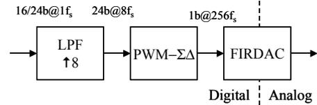
Figure 19. PWM  $\Sigma\Delta$  FIRDAC
