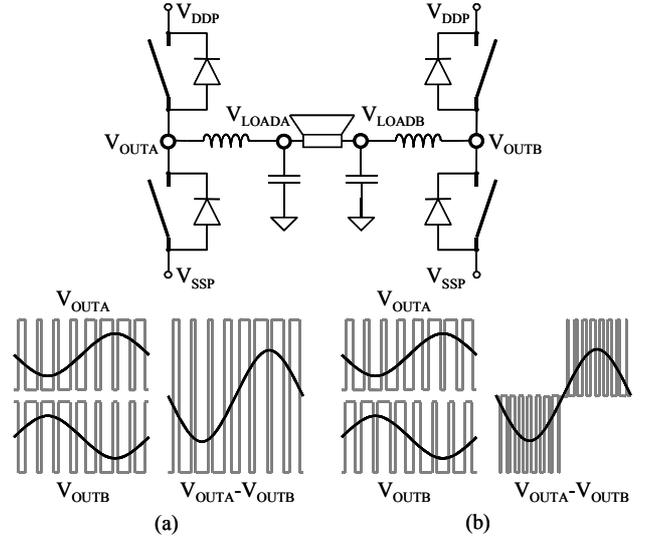
Figure 6. BTL configuration with (a) AD modulation (b) BD modulation.
