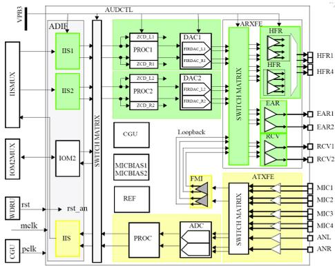
Figure 16. Audio codec in typical ABB system.
