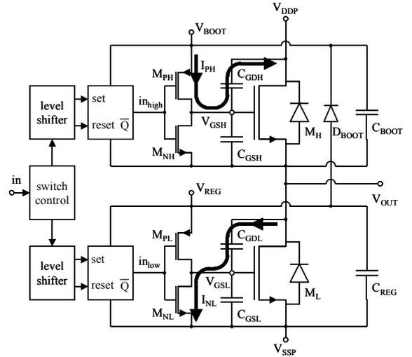
Figure 12. Typical class-D output stage configuration.
