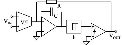
Figure 10. Hysteretic self-oscillating class-D feedback loop.
