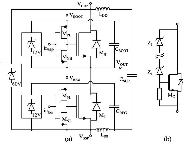
Figure 14. (a) parasitic inductances and voltage clamping (b) active clamp
