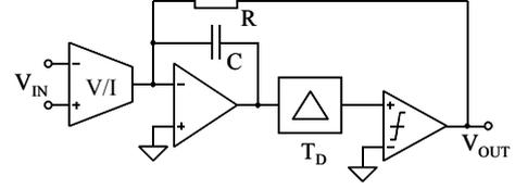
Figure 9. Delay based self-oscillating class-D feedback loop.
