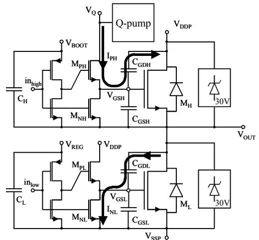
Figure 15. Automotive class-D output stage
