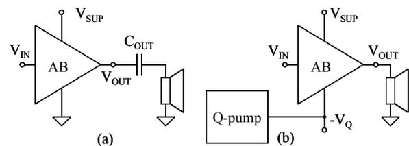
Figure 18. Headphone amplifiers (a) AC coupled (b) True ground
