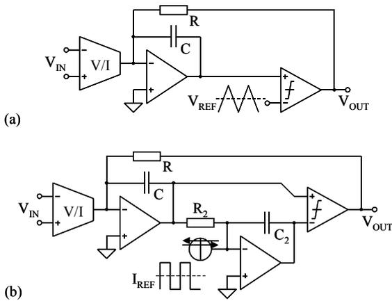
Figure 11. Fixed-Carrier class-D feedback loops (a) 1<sup>st</sup> order (b) 2<sup>nd</sup> order.
