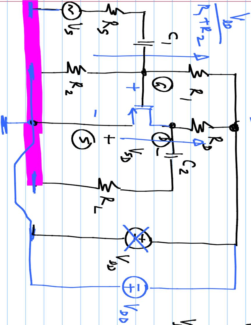
$$\frac{\mu_n C_{ox} W}{2} (V_{GS} - V_T)^2$$
