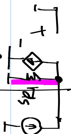
$$R_{\text{out}} = \frac{1}{g_{mV_{DS}}} + \cancel{\frac{1}{h_{fe}}(1+g_{mV_{DS}}) \cdot r_{ds}} \cdot R_L$$
