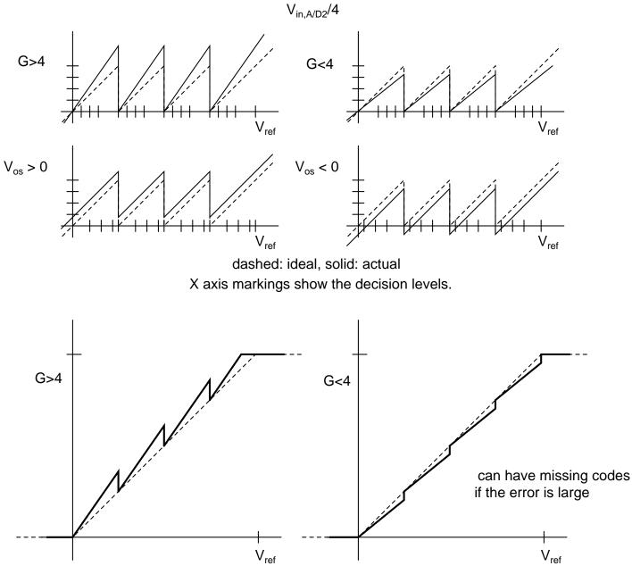
A/D characteristics shown as a transfer curve(straight line passing through the steps) They can be similarly generated for the case with offsets
