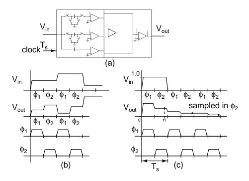
Figure 1: (a) A general switched capacitor filter, (b) General form of inputs and outputs, (c) Setup for impulse response simulation (input changes with **rising edge of**  $\phi_1$  and the **output is taken in**  $\phi_2$ )
