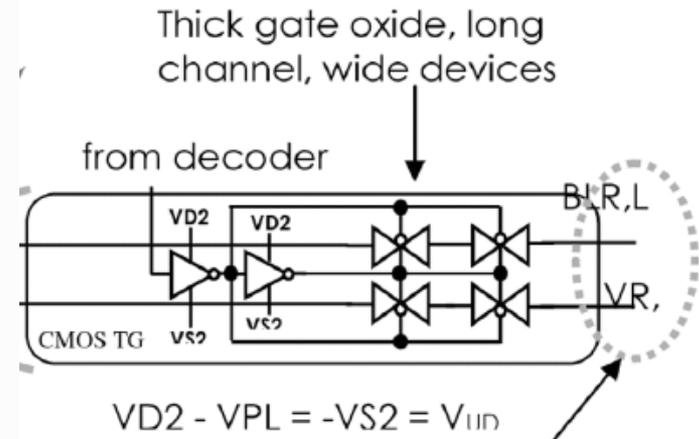
For unselected cells, under-drive pass gates to reduce leakage noise
