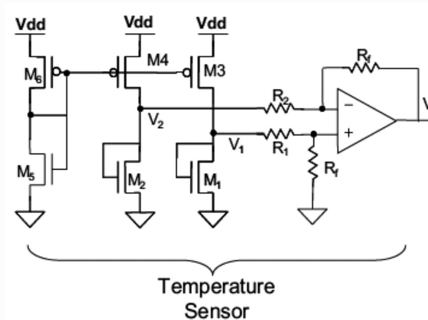
Leakage is exponential function of temperature
