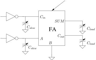
Use parasitic extracted netlist for simulation
