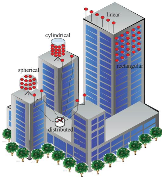
Fig. 26. Typical antenna array configurations and deployment scenarios of LS-MIMO systems [569].
