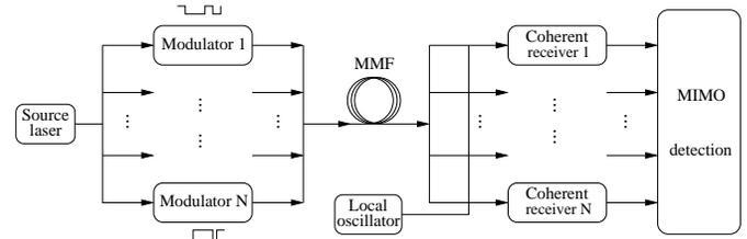
Fig. 31. An example of MIMO optical fiber system.
