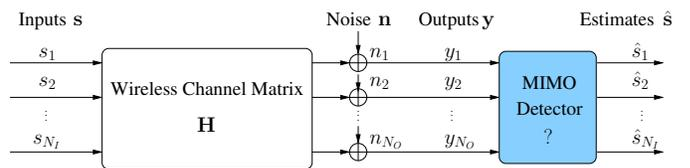
Fig. 4. Conceptual illustration of the MIMO detection problem.
