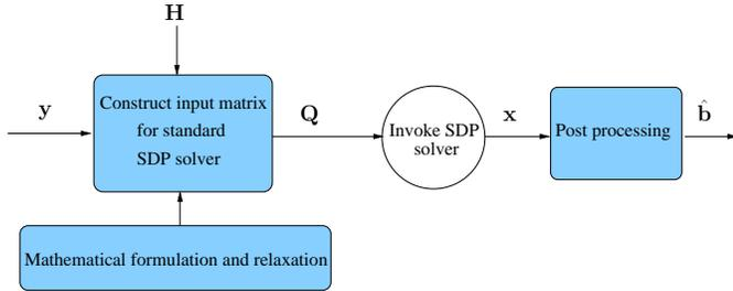
Fig. 25. The basic principle of the SDPR based MIMO detectors.
