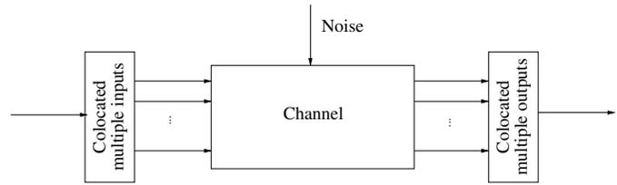
Fig. 8. Point-to-point MIMO channel.
