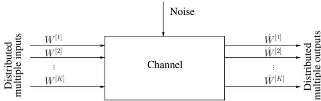
Fig. 11. MIMO interference channel, where  $W^{[k]}$  represents the message that originates at transmitter  $i$  and is intended for its dedicated receiver  $i$ , while  $\hat{W}^{[i]}$  denotes the recovered version of  $W^{[k]}$ ,  $k = 1, \dots, K$ .
