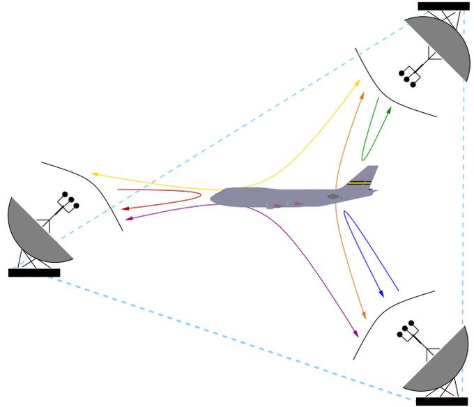
Fig. 30. Conceptual illustration of MIMO radar systems.
