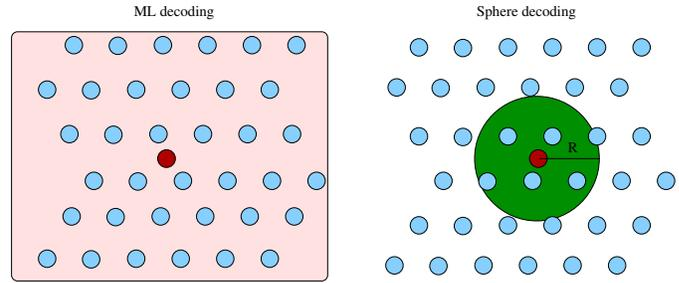
Fig. 22. The basic principle of the SD based MIMO detectors. In short, it solves the problem of finding the “closest” lattice point to a given vector  $y$  in the skewed and rotated (caused by the MIMO channel) lattice  $Hs$ .
