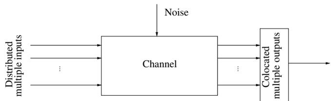
Fig. 9. MIMO multiple-access channel.
