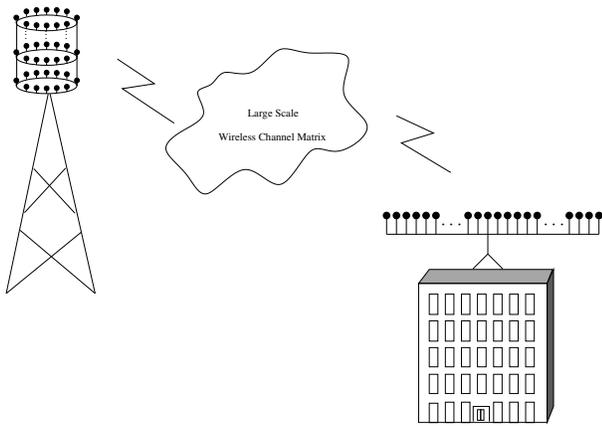
Fig. 27. An example of Type-I (point-to-point) LS-MIMO systems.
