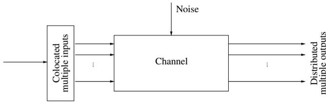
Fig. 10. MIMO broadcast channel, which is not suitable for MIMO detection.
