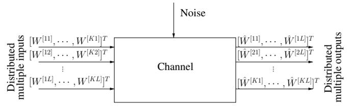
Fig. 12. MIMO X channel, where  $W^{[kl]}$  represents the message that originates at transmitter  $l$  and is intended for receiver  $k$ , while  $\hat{W}^{[kl]}$  denotes the recovered version of  $W^{[kl]}$ ,  $k = 1, \dots, K$ ,  $l = 1, \dots, L$ .
