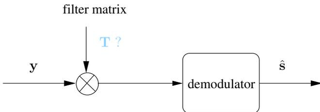
Fig. 19. Conceptual illustration of linear MIMO detectors.
