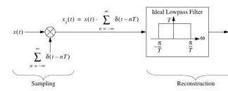
In the sampling process, x(t), the signal to be sampled, is multiplied by the impulse train, yielding the sampled signal  $x_s(t)$ . In order to perform reconstruction, we pass  $x_s(t)$ through the ideal lowpass filter, yielding the reconstructed signal  $x_{sr}(t)$ .
