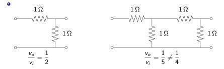
• Beware of loading! If the two sections are connected through a voltage-follower, overall transfer function will be  $\frac{1}{4}$
