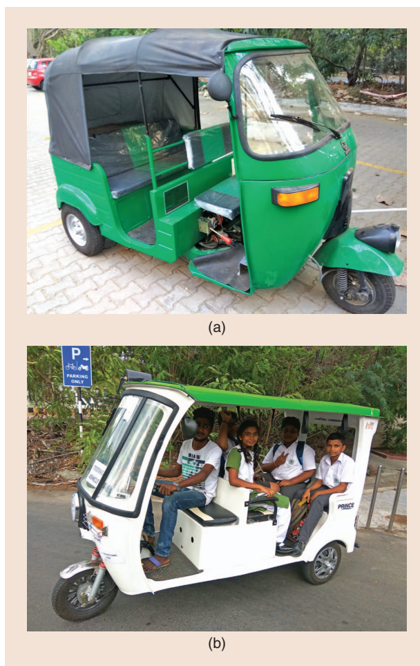
Figure 2. (a) An electric auto (the most widely used example of a general three-wheeler) and (b) an electric rickshaw.
