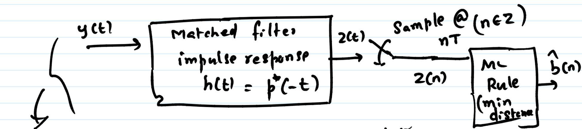
Optimal demod for stream of symbols when delayed pulses  $p(t-nT)$  are orthonormal
