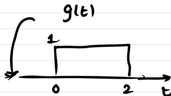
delayed pulses are orthogonal (no ISI)
