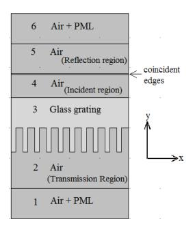
**Figure 2.** 2-D geometry describing the various domains of the one dimensional binary phase grating model.
