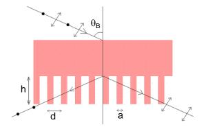
**Figure 1**. 2-D view of a grating that splits TE and TM components into different orders. h,n - height and refractive index of the grating, d - period, a/d - fill factor, and  $\theta_{\rm R}$  - incident Bragg angle.
