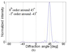
**Figure 6.** Transmitted far E-field distribution for PBS-B design at Bragg incidence of 45° with plots of (a) TE component and (b) TM component
