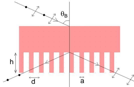
**Figure 1.** 2-D view of a grating that splits TE and TM components into different orders.  $h, n$  - height and refractive index of the grating,  $d$  - period,  $a/d$  - fill factor, and  $\theta_B$  - incident Bragg angle.
