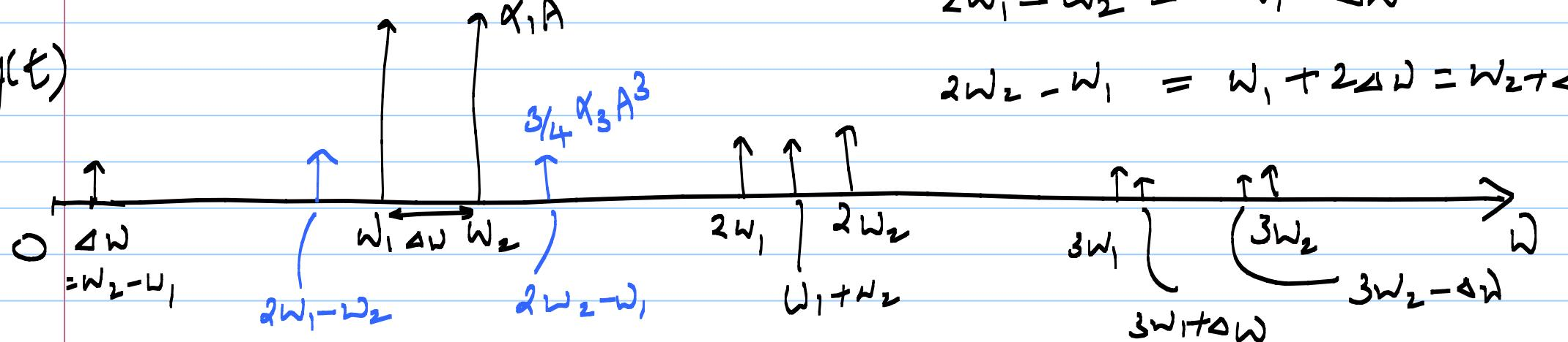
$\text{Im}_3$  components @  $2\omega_2 - \omega_1$  &  $2\omega_1 - \omega_2$
